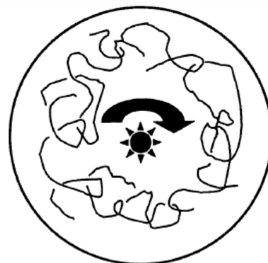
Figure 10.20 Molecular forces involved in the Weissenberg effect. Note polymer orientation and entanglements.
