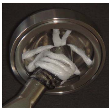
Fiber-hinge with rotational freedom in various directions, designed as a potential hip joint implant. The inside view shows 3 white cable pairs to the "equator" and one black cable to the "pole" of the cup.
