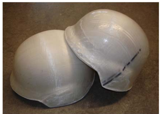
Figure 7. Two helmet shells made by creep-forming of gel-spun UHMWPE fibers [14].
