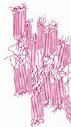
4. Separation of crystalline block segments during the third stage
